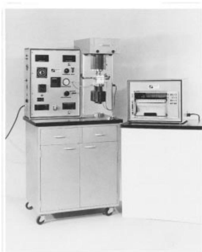
FIG. 3 Failex Variable-Speed Four-Ball Wear Test Machine
